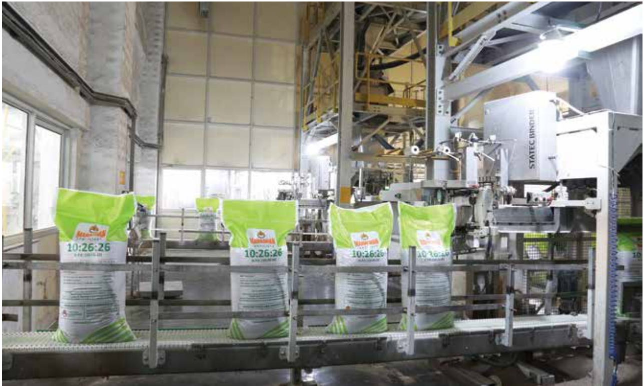
NPK bagging plant at Taloja
